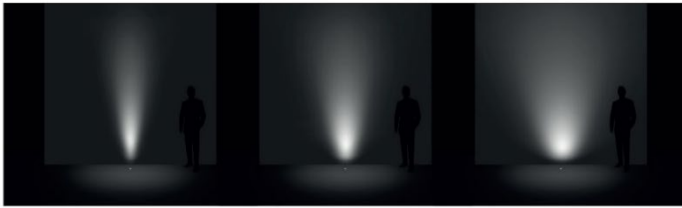
Flood: 30° Medium Flood: 45° Medium Flood: 60°
